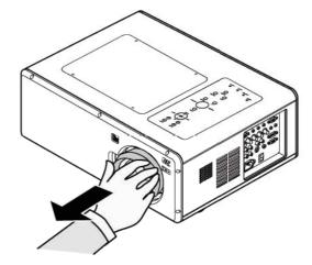
Push the LENS RELEASE button all the way in and rotate the lens counterclockwise.
